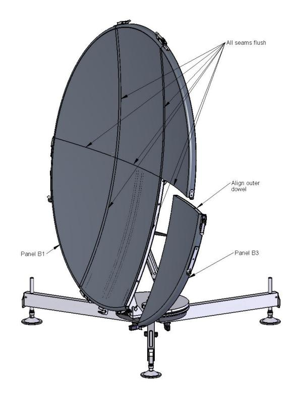
After making sure all seams look flush fasten the two latches on the back of the dish, then fasten the six remaining perimeter latches.
